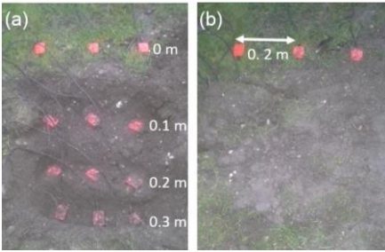
Figure 1: Geophone configuration used to test the effects of geophone burial on rain noise before (a) and after (b) burial and compaction.
