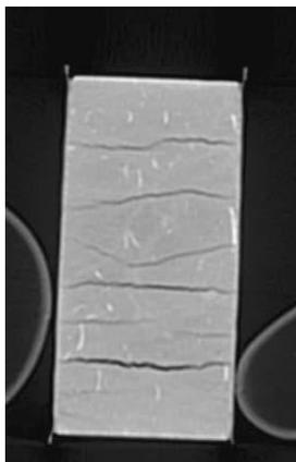
**Figure 2: Horizontal bands resulting from vertical compression of a calcarenite.**
