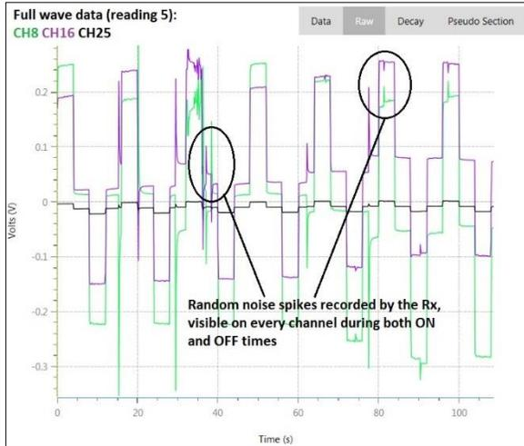
**Figure 3: Full wave data (reading 5, channels 8, 16 and 25) from a survey reading heavily affected by noise.**
