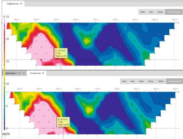
For example, a Newmont standard chargeability can be recalculated from an arithmetic dataset by integrating time windows from 450ms to 1,100ms. Figure 6 presents the original chargeability pseudosection with the arithmetic window scheme for 2-second time base survey against the re-processed pseudosection using the Newmont scheme.
