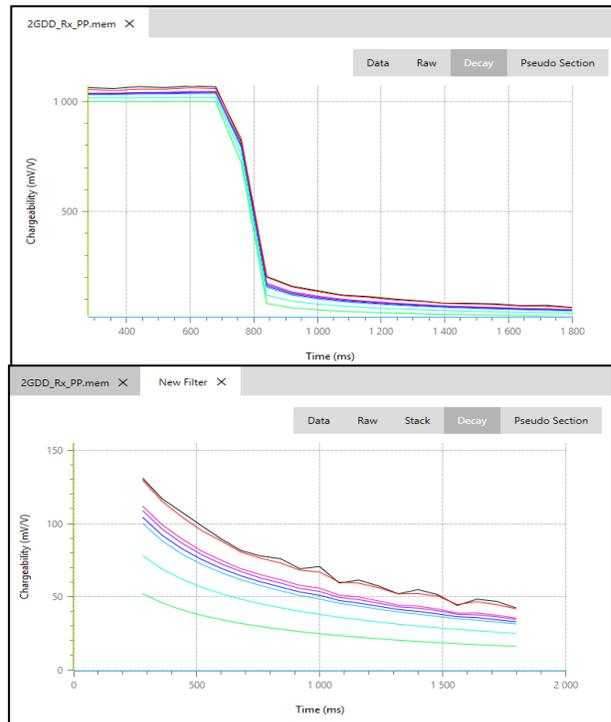
**Figure 5: (Top) Original decay with timing error resulting in an over-estimated chargeability value of 400 mV/V, (Bottom) Resulting decay from fixed timing between Tx and Rx with chargeability value of 65 mV/V.**
