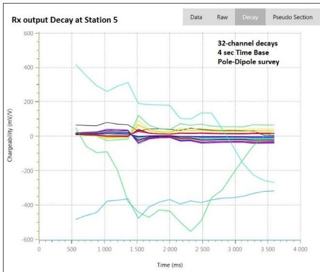
**Figure 2: Original decays (reading 5) heavily affected by noise.**
