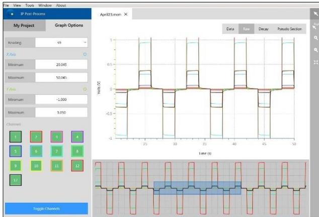
**Figure 1: Example of full wave data from a Pole-Dipole survey (a=10m, n=1-16).**
