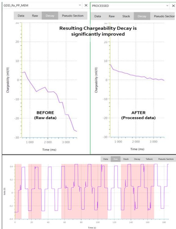
**Figure 4: (Top) Discarded noisy half-cycles of reading 2, in red. (Bottom) Original noisy decay (left) vs post-processed decay (right).**
