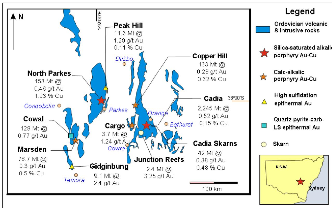
Figure 1. Porphyry copper-gold deposits in Macquarie arc belt, after Cook et al., 2009.
