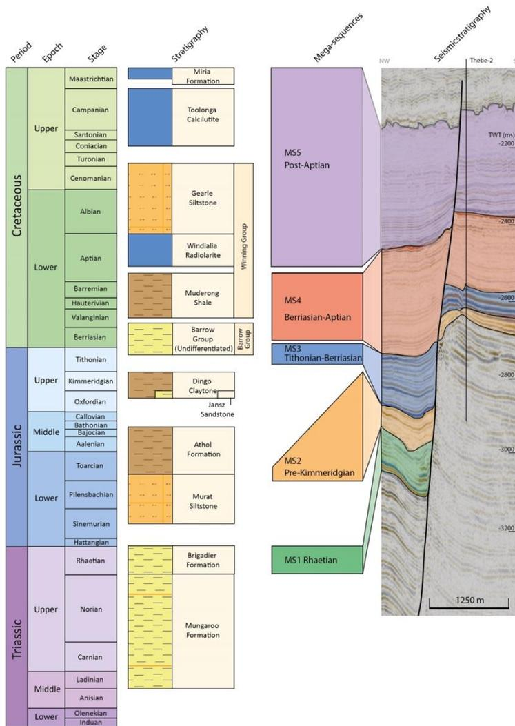
**Figure 3 Generalised stratigraphic column for the Exmouth Plateau, with the authors mega-sequence framework constrained to a seismic inline from the Thebe 3D survey.**
