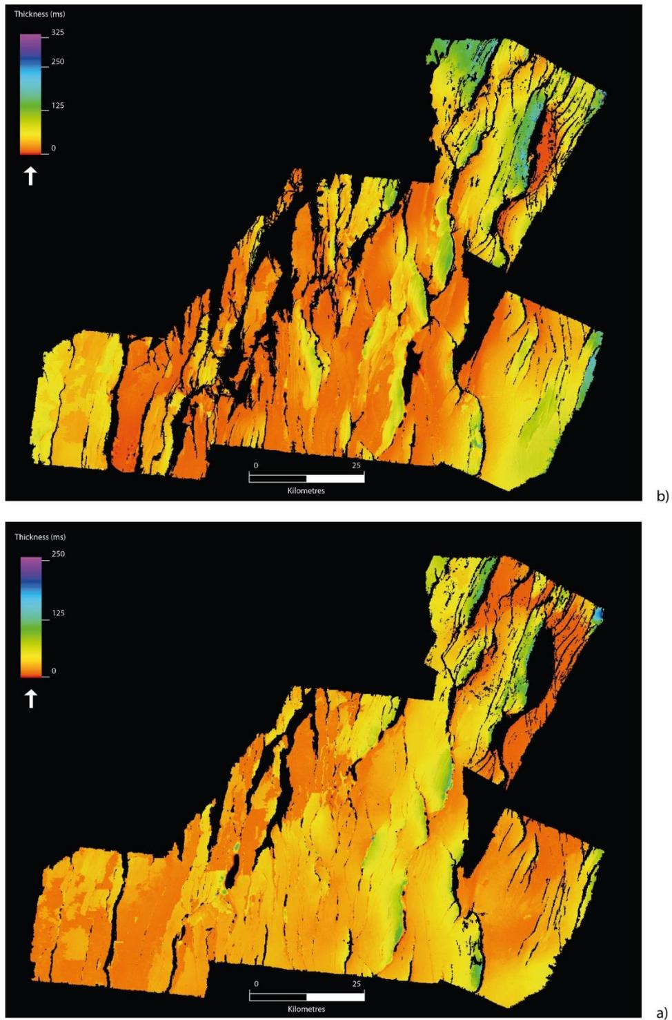
**Figure 4 Thickness maps of (a) MS1 Rhaetian and (b) MS2 Pre-Kimmeridgian in the central Exmouth Plateau.**
