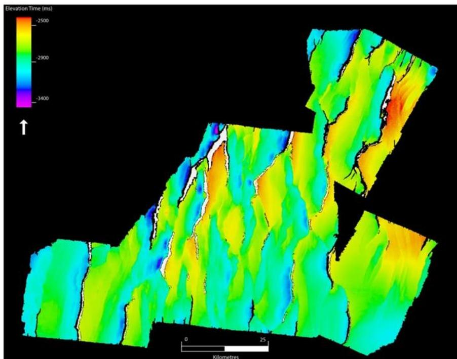
**Figure 5 Rift-related architecture of the study area, shown on the top Norian-Mungaroo Formation surface. Eroded fault block crests are displayed in white.**
