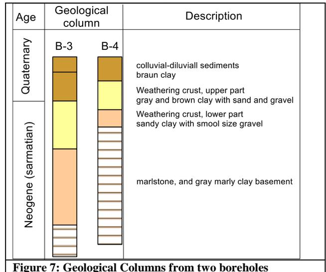
**Figure 7: Geological Columns from two boreholes**
