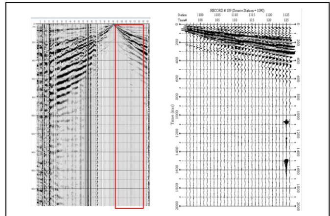
Figure 6: Selection of 31 traces for MASW analysis from a shot record collected for reflection processing.
