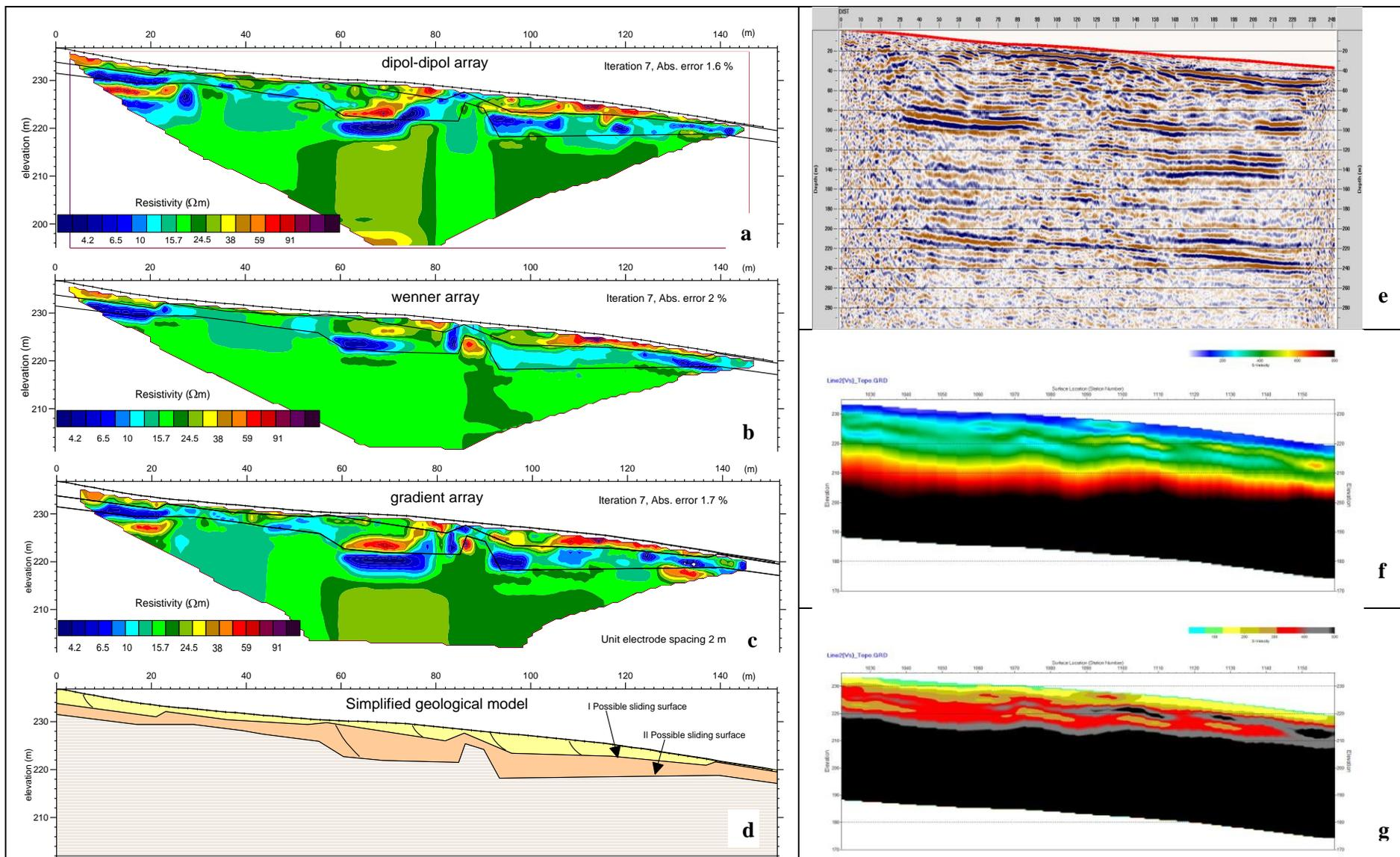
Figure 8: Line 2- (Left) Three different electrode arrays were used in resistivity measurement. a) dipole-dipole; b) Wenner and c) multiple gradient; d) Geological interpretation from cooperative inversion seismic-resistivity data. (Right) e) DMO section; f) Vs section by MASW; g) Vs section blocked at every 50m/s.
