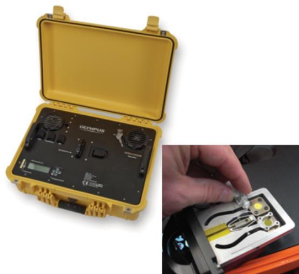
Figure 2: The Olympus Terra portable XRD instrument (left image) and the vibrating sample (right image).
