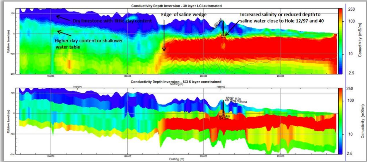
Figure 3. Line 201201 LCI and SCI section. Thick red zone represents the saline wedge.
