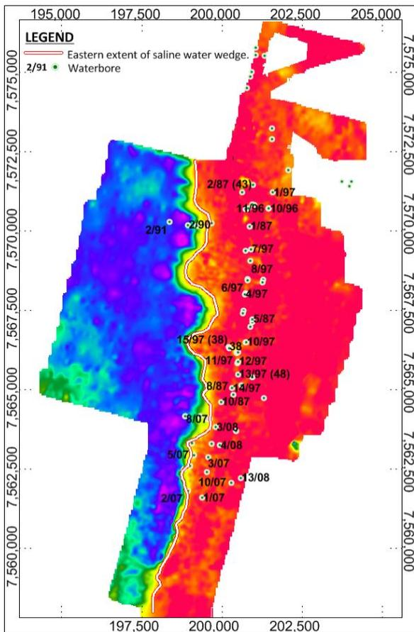
**Figure 2: Interpreted edge of Seawater interface on -43m (AHD) LCI.**
