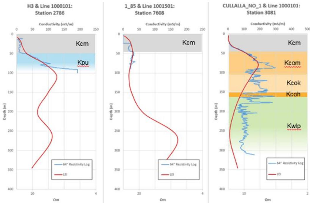
Figure 2: Wireline borehole conductivity (blue line) with drilled lithology information (coloured box). AEM LEI data is superimposed in red. Kpu – Upper Parmelia (sandstone with basal siltstone which acts as aquitard); Kcm – Molecap Greensand surficial sediment; Kcok Mirrabooka Member silty, poorly-sorted sandstone; Kcok Kardinya Shale; Kcoh Henley Sandstone; Kwlp – Pinjar Member of the Leederville Formation. The right-most image is the Cullalla\_NO\_1 borehole shown in Figure 3.
