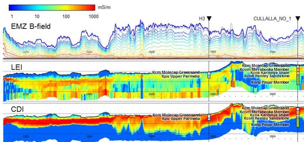
Figure 3: Tempest 75 Hz data (top) along with layered earth inversion model (middle) and EMFlow conductivity depth image (bottom). The borehole lithology log has been superimposed with colour denoting a different lithology, not conductivity.
