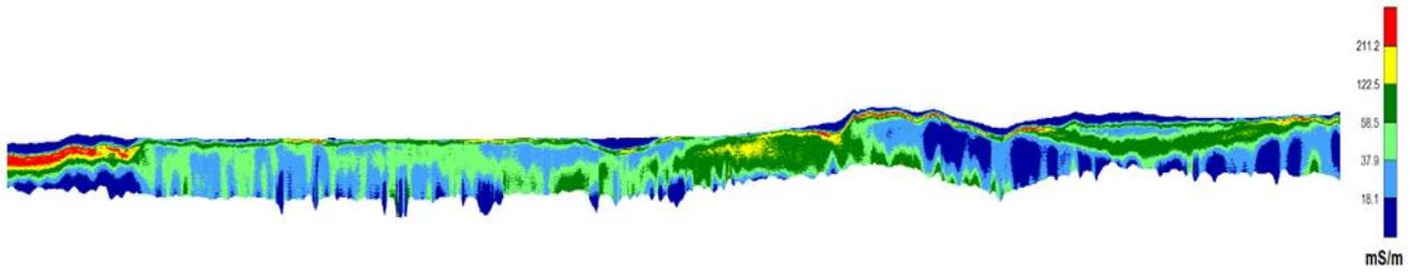
**Figure 4: Conductivity depth section (EMFlow) with the colour intervals corresponding with amount of total dissolved solids in a sandy formation (providing an indication of water quality), ranging from brackish (red) to fresh (blue).**
