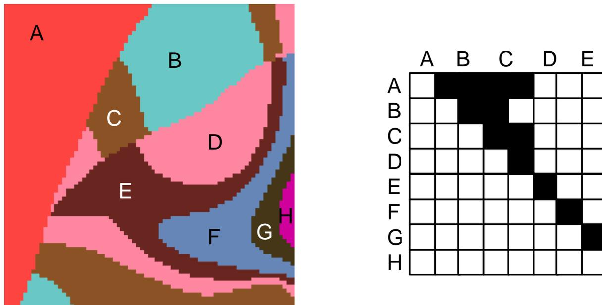
**Figure 1: Raster geological map (left) and equivalent Adjacency Matrix (right) showing neighbourhood relationships for each lithological unit. In this case the calculation simply returns a Boolean “are neighbours” (black) or “are not neighbours” (white). The calculation can be performed on raster maps, as shown here) or polygonal GIS files, the only difference being the limits to resolution of individual pixels and the spacing between nodes in the two cases.**
