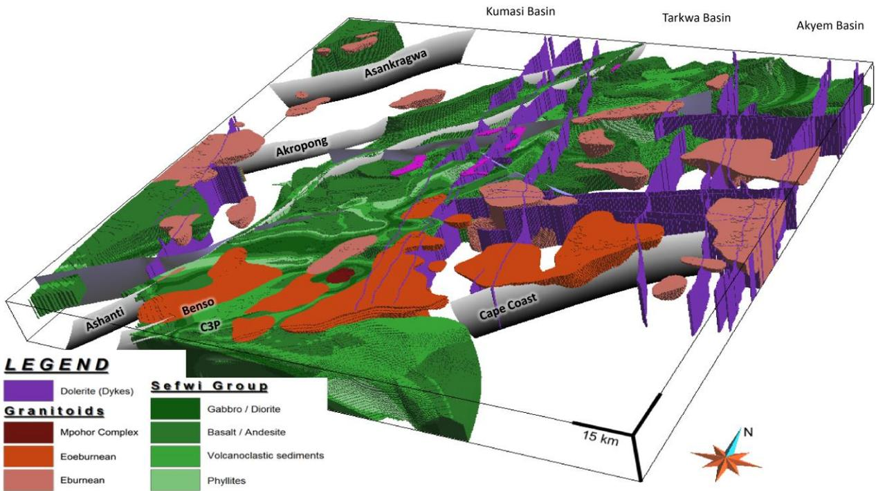
Figure 2: 3D geological model of South West Ghana based on field observations, prior mapping and gravity inversions (after Perrouty et al, 2014). The full 23 lithological units are here simplified to 8 visible units with the others made transparent to aid visualisation. The faults were used to build the model but are not considered in this study.
