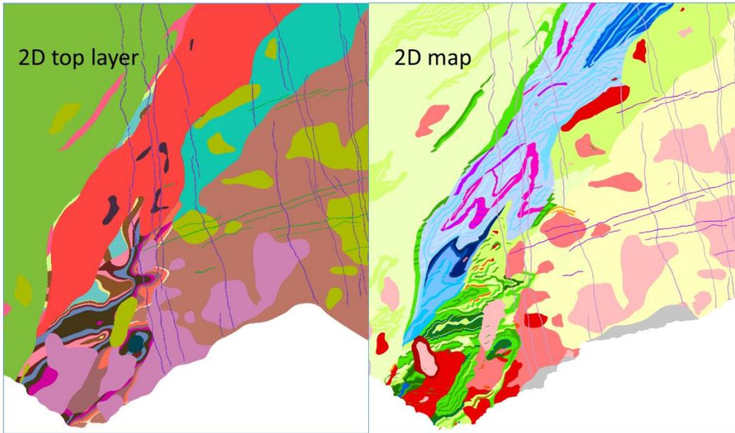
Figure 4 Comparison of the top layer of the 3D geological model (left) and the 2D geological map compiled for the same area, which retains significantly more detail than were able to maintain in the 3D model. Each map is 160 km across.
