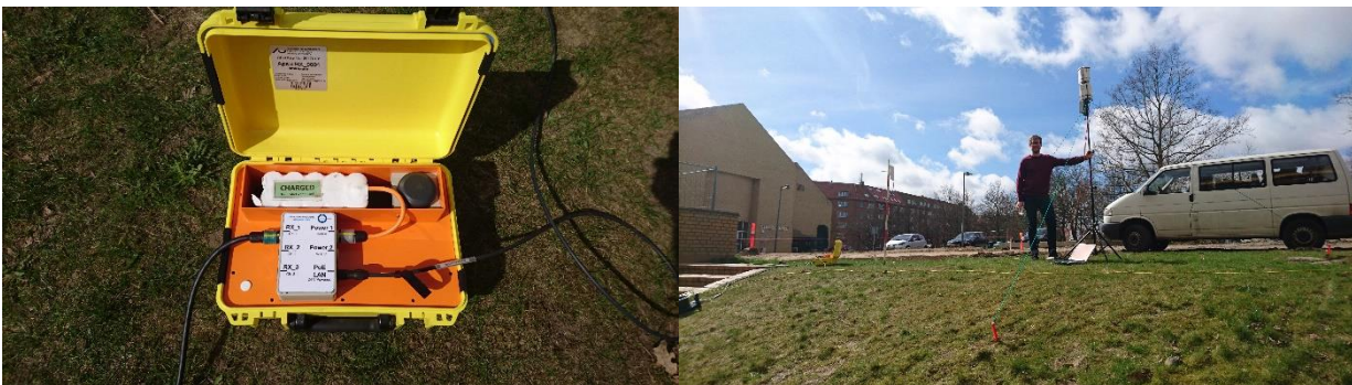
Figure 2: Photos of the surface NMR receiver system. Left: A 3-channel receiver box powered by battery at the top left. The round dark gray unit at the top right is the GPS antenna. Right: The mast with the WiFi antennas. To obtain full 360° coverage 8 individual antennas are used. A receiver box is seen at the left side of the photo.
