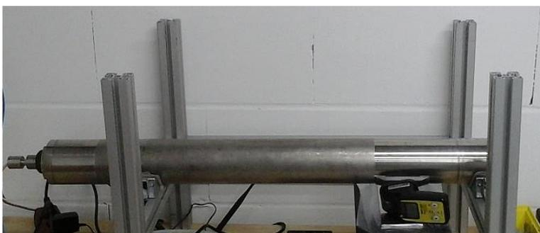
**Figure 1: Prototype 125 mm blasthole XRF probe during bench testing.**
