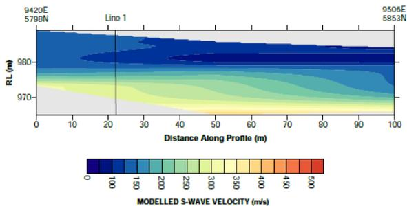
**Figure 4: Line 3 2D profile showing the variations of Vs within the subsurface. The line starts in the west and ends in the east.**
