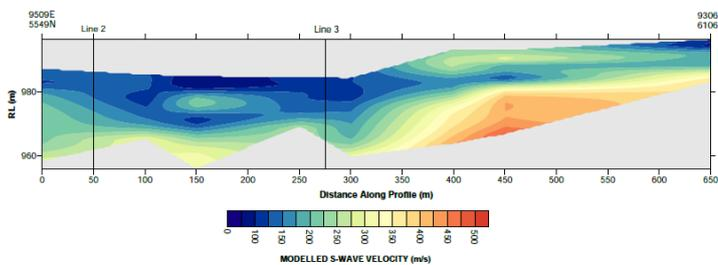
**Figure 2: Line 1 2D profile showing the variations of Vs within the subsurface. The line starts in the south and ends in the north.**
