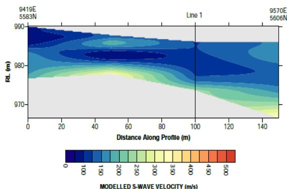
**Figure 3: Line 2 2D profile showing the variations of Vs within the subsurface. The line starts in the west and ends in the east.**
