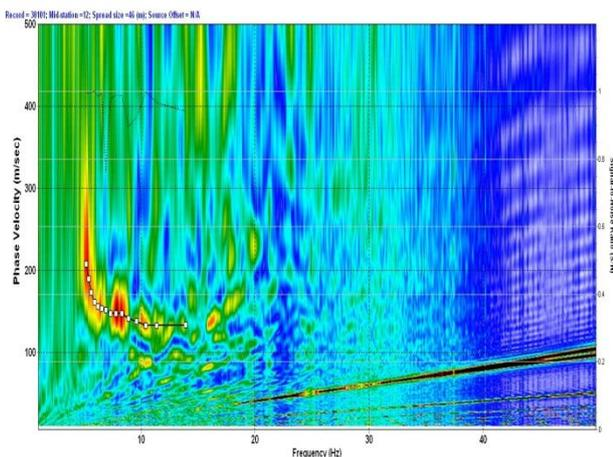
**Figure 1: Example Dispersion curve from Line 3 showing a fundamental curve between 5 Hz to 15 Hz.**
