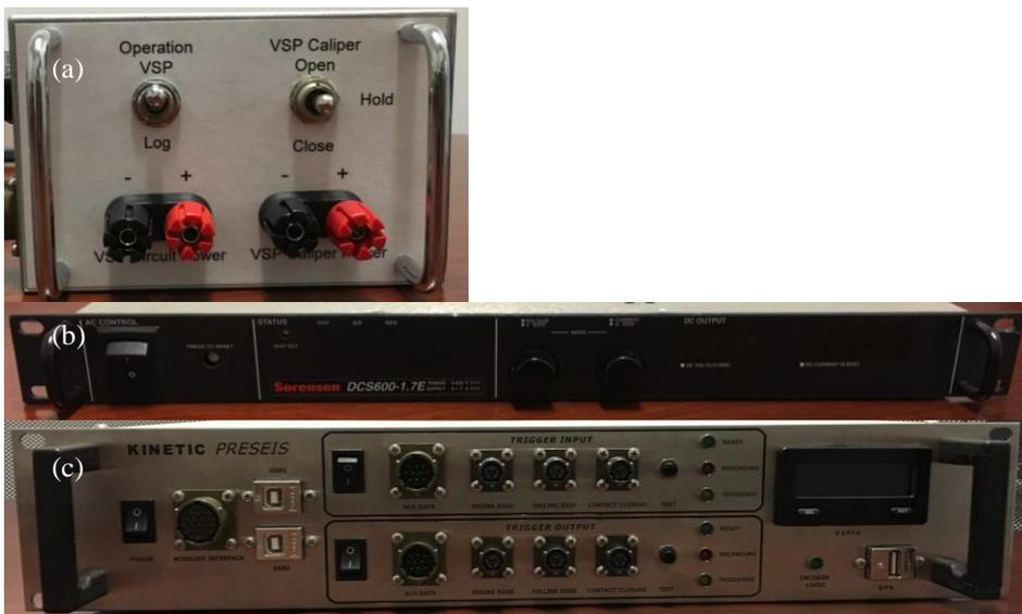
**Figure 8: VSP System components: (a) Tool caliper control, (b) power supply, (c) seismic interface box.**
