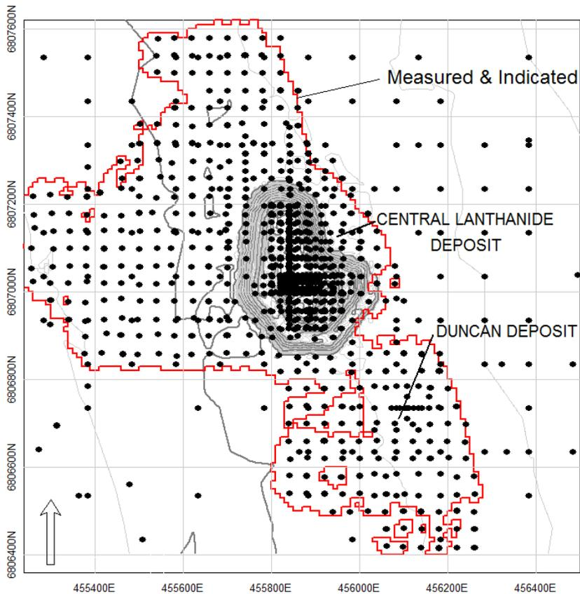
**Figure 4. Mt Weld, drilling plan for the 2008 resource estimate**
