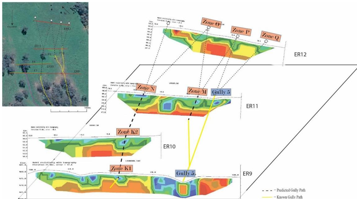
**Figure 4.** Integrated ERI results with an associated Google Earth image for site C; depicting the interpreted LPP shown as the black dashed line which intersects each profile through a shallow conductor.
