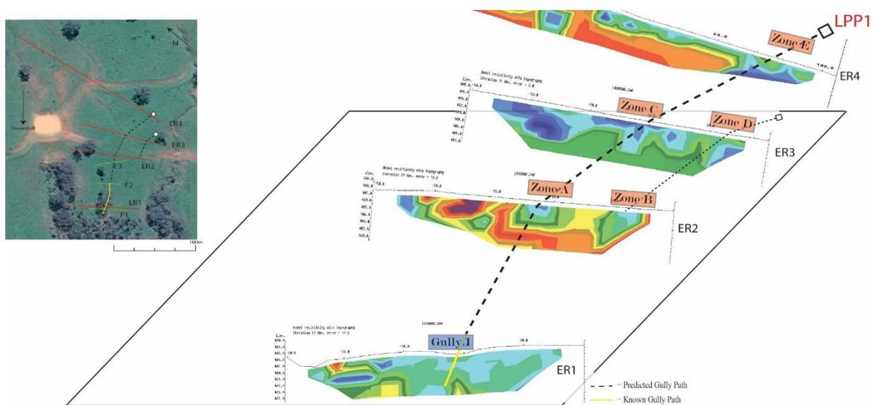
**Figure 3.** Integrated ERI results with an associated Google Earth image for site A; positions and orientations of each profile are relative to on ground positions shown as the small image to the top left of the figure.
