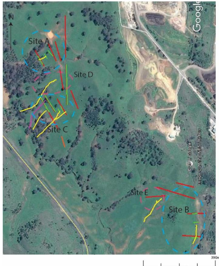
**Figure 2.** Image depicting the positions of all electrical resistivity (shown as solid red lines), FEM (shown as solid green lines) surveys and identified surface expressions of gullies (shown as solid yellow lines) across the site. Primary sites are represented by blue dashed circles and labelled as A, B, C. Secondary sites are depicted as pink dashed circles and labelled as D and E. Orange line depicts ERI survey conducted for background readings.
