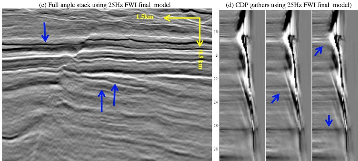
Figure 4: Kirchhoff PSDM stack and CDP gathers. (a) and (b) are migrated results using tomography model (FWI input). (c) and (d) are migrated results using 25Hz FWI model.
