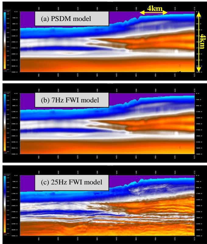
Figure 3: Velocity model panels (a) final PSDM model. (b) and (c) are the 7Hz and 25Hz FWI results.
