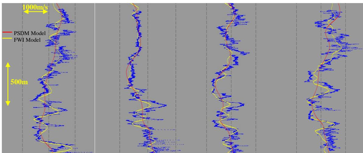
Figure 6: Sonic log comparisons for four separate wells
