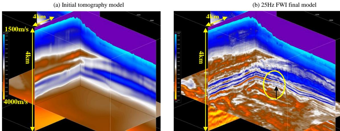
Figure 5: 3D model view: (a) Initial tomography model. (b) 25Hz FWI model.
