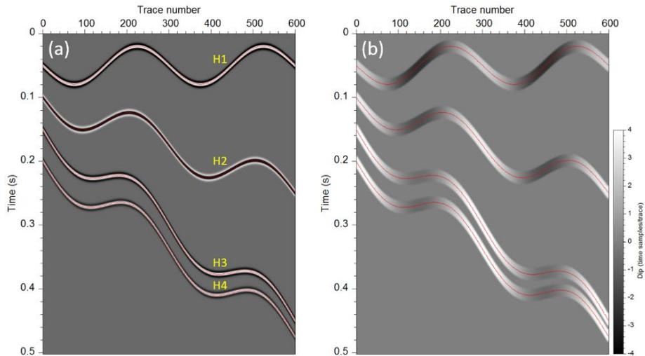
Figure 1 Local seismic dip estimation: (a) a synthetic seismic section with 4 reflection events in variable dips; (b) Estimated local dips for the seismic events in (a). The red curves are the time picks for the 4 reflections.
