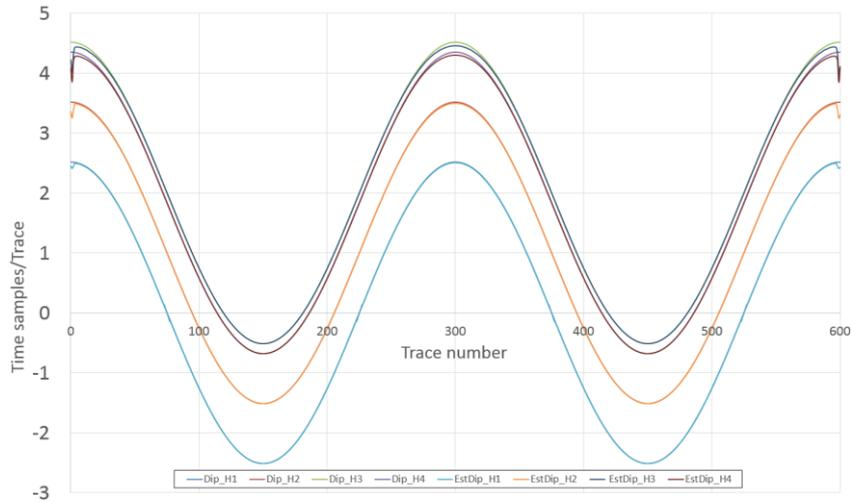
Figure 2 The comparison of the estimated local dips (EstDip\_H1, EstDip\_H2, EstDip\_H3 & EstDip\_H4) by equation (3) with the corresponding true dips (Dip\_H1, Dip\_H2, Dip\_H3 & Dip\_H4) of the 4 horizons (H1, H2, H3, & H4) in Figure 1.
