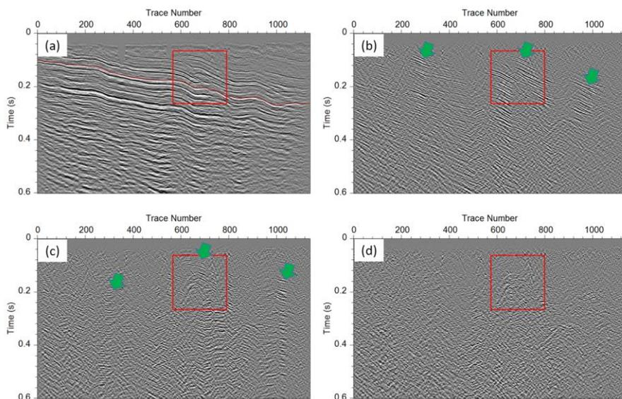
Figure 3 Diffraction extractions by with a 21-trace MAEF filter: (a) Original seismic stack section overlaid with a picked reflection in red curve; (b) extracted by a direct application of the MAEF filter to the section in (a); (c) Created by applying the MAEF filter to the flattened section of (a) with the picked reflection followed with restoring the flattening process; (d) Obtained by applying the MAEF filter in the local dip direction estimated by equation (3).
