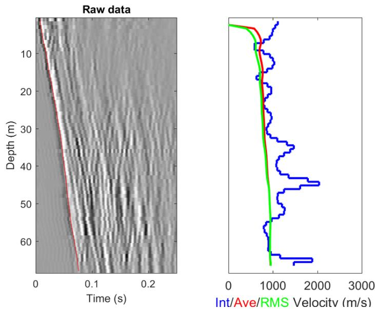
**Figure 7: (left) raw data and (right) extracted velocity profiles. Multiple reflections can be seen on the raw data (events going from the bottom left to the top right of the plot). The average velocity is each depth divided by the time taken to reach that depth from the surface ( $\sum_{i=1}^n V_i t_i / \sum_{i=1}^n t_i$ ). RMS velocity is given by  $\sqrt{\sum_{i=1}^n v_i^2 t_i / \sum_{i=1}^n t_i}$ .**
