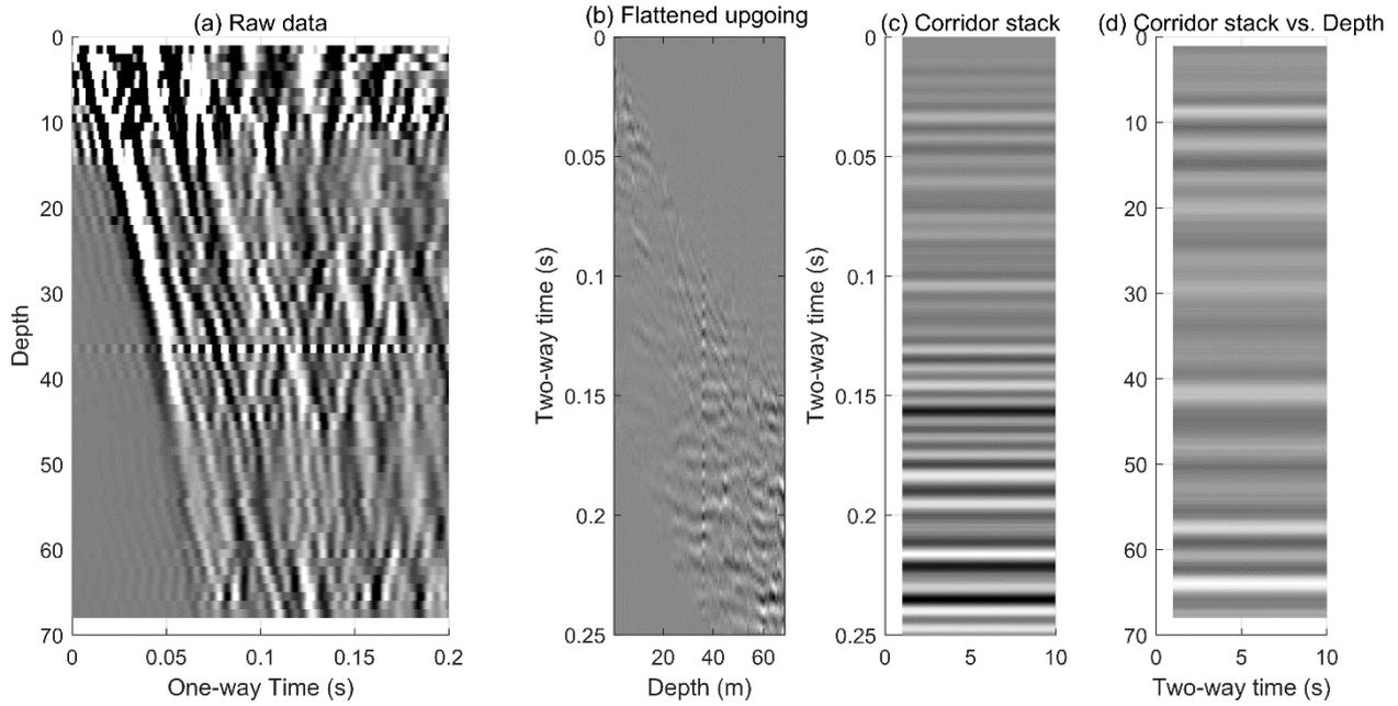
**Figure 8:** An example of data that has been processed through to corridor stack. Note that the flattened up-going events are shown prior to the application of the mute.
