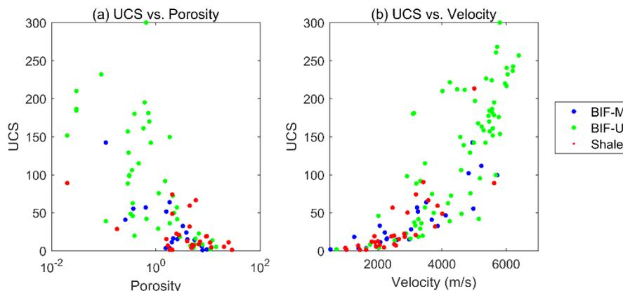
**Figure 1: The relationship between uniaxial compressive strength and porosity and p-wave velocity.**
