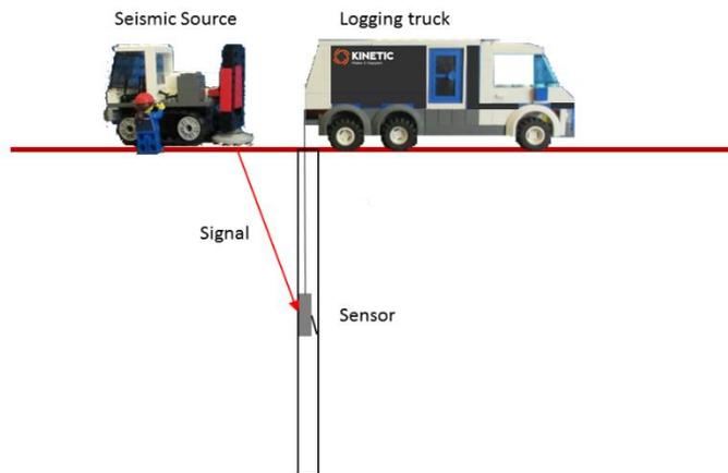
**Figure 4: Simplified diagram of VSP acquisition.**
