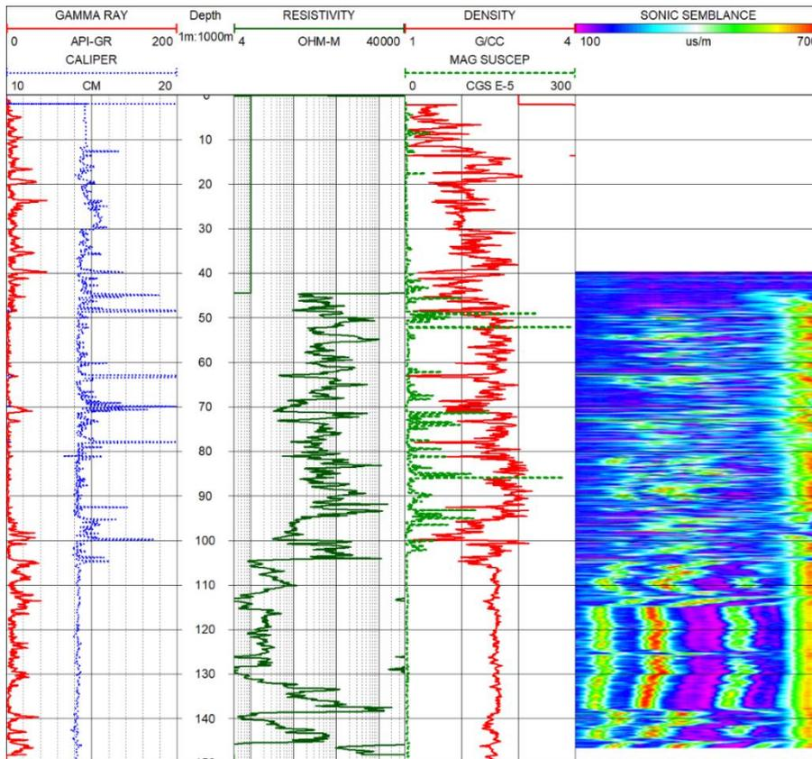
**Figure 3: A typical downhole geophysical dataset recorded in the Pilbara. Note the strong arrivals in the competent formation from 115 to 150m, but the weak and inconsistent signals in the more friable formations above 115m. Note the calliper signifying rugose hole conditions in the upper part of the hole and the water level at around 44m.**
