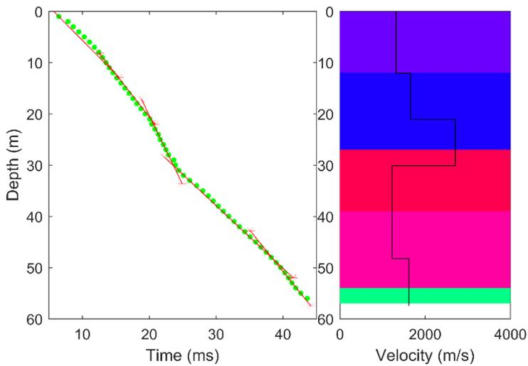
**Figure 9:** Left: First-break picks (green dots) and fitted velocities (red lines). Right: Resulting interval velocities overlain on the logged geology.
