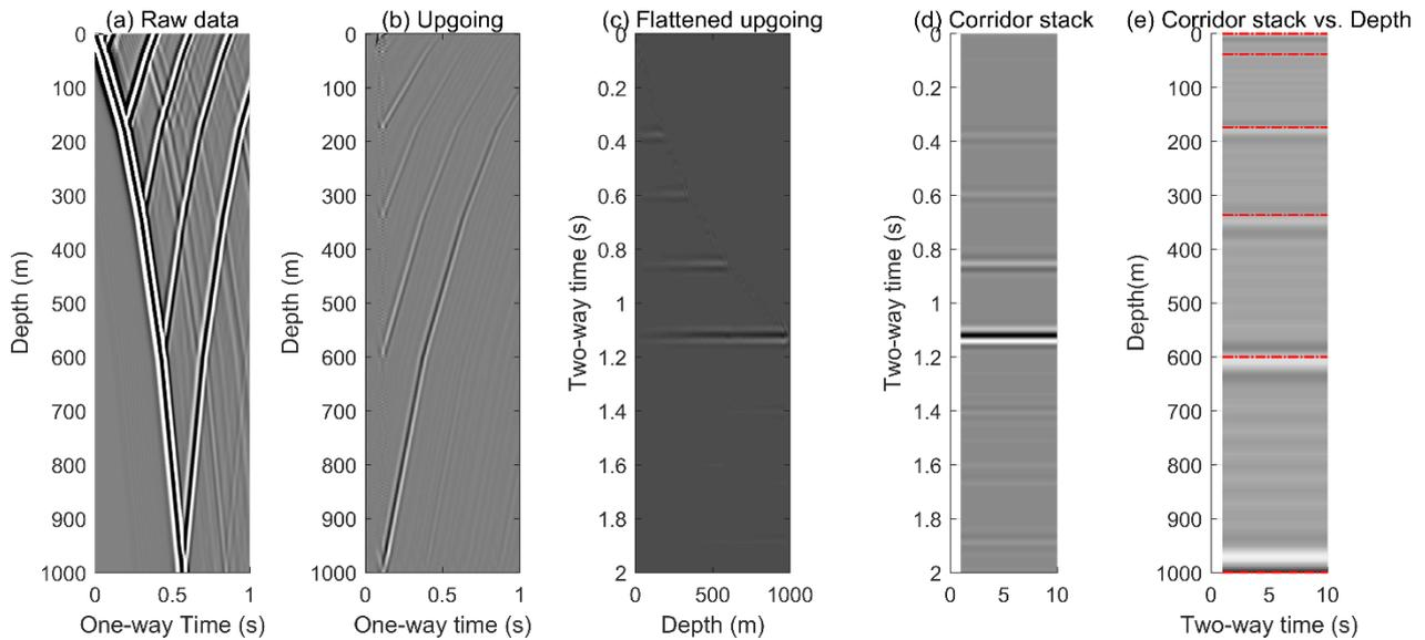
**Figure 6: Modelled data at various stages in processing. The red lines on (e) indicate the actual depths of the interfaces in the model.**
