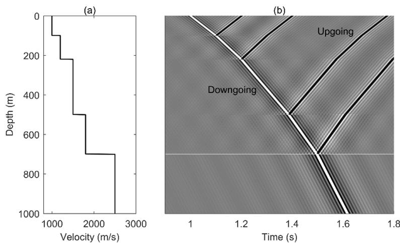
**Figure 5: Synthetic VSP record. The down-going and up-going (reflected) wavefields are labelled on (b).**
